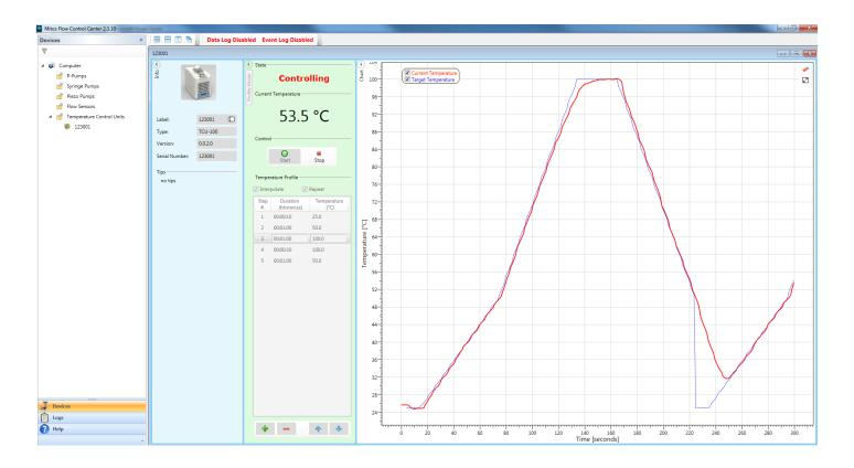
A screenshot of the Flow Control Centre software showing the interpolate function, which allows the user to perform controlled temperature ramps
