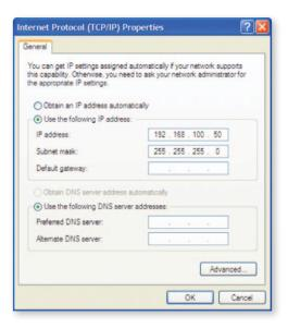
**Step 4.** Select "Use the following IP address" and enter 192.168.100.50 for the IP address and 255.255.255.0 for the Subnet mask. Press the OK button and close all open dialog boxes so the settings take effect.
