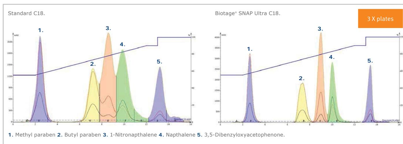
**Figure 2.** Comparison between standard C18 flash cartridges and Biotage® SNAP Ultra C18. Solvent A (water), B (methanol); Gradient 55% B for 2CV, 55–90% B for 10CV, 90% B held for 1CV then 100% B for 3CV (1% sample load, 300 mg sample).
