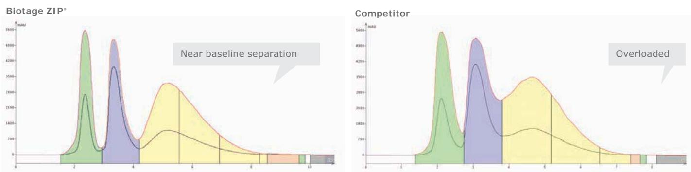
**Figure 6.** A 30 g Biotage ZIP® cartridge (left) and a competitive 30 g flash cartridge with spherical silica (right) are used to isocratically separate a 3-component mix. The Biotage ZIP® cartridge provides more compound resolution and sharper peaks for the same sample load.
