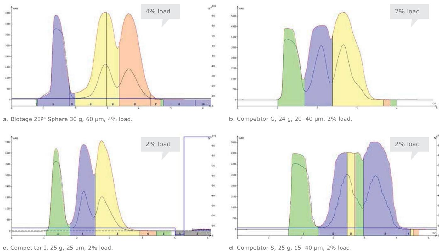
**Figure 5.** During the testing, a Biotage ZIP® Sphere cartridge (a) with a 4% sample load (1.2 g) provided a separation equivalent or better than three competitive 25 g/25 µm silica cartridges (b–d) each loaded with a much smaller 2% sample load (0.5 g).
