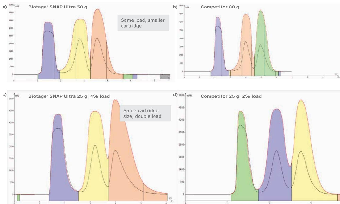
**Figure 1.** The very high surface area of the spherical 25 µm Biotage® HP-Sphere™ silica enables the use of smaller cartridges for the same amount of sample. In these examples, a Biotage® SNAP Ultra 50 g cartridge (a) actually purifies more sample than a competitive 80 g high-performance cartridge (b), saving 38% solvent and run time.
