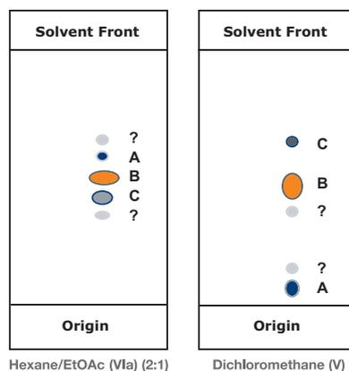
**Figure 12.** Impact of solvent selectivity on a chromatographic separation. In hexane/ethyl acetate the compound of interest (B) is poorly resolved from its major impurities (A and C). In dichloromethane, retention of impurities A and C has been dramatically altered, providing a better purification of B.
