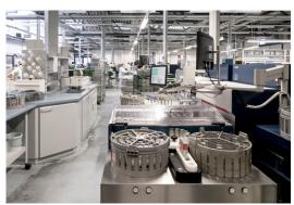
Based on Individual Bacteria Count (IBC), BactoScan™ FC+ gives an accurate determination of the hygienic quality of raw milk with a capacity of testing up to 200 samples per hour. BactoScan is the industrial standard in many countries all over the world, and in the EU more than 75% of all milk supplies are paid based on BactoScan results.
