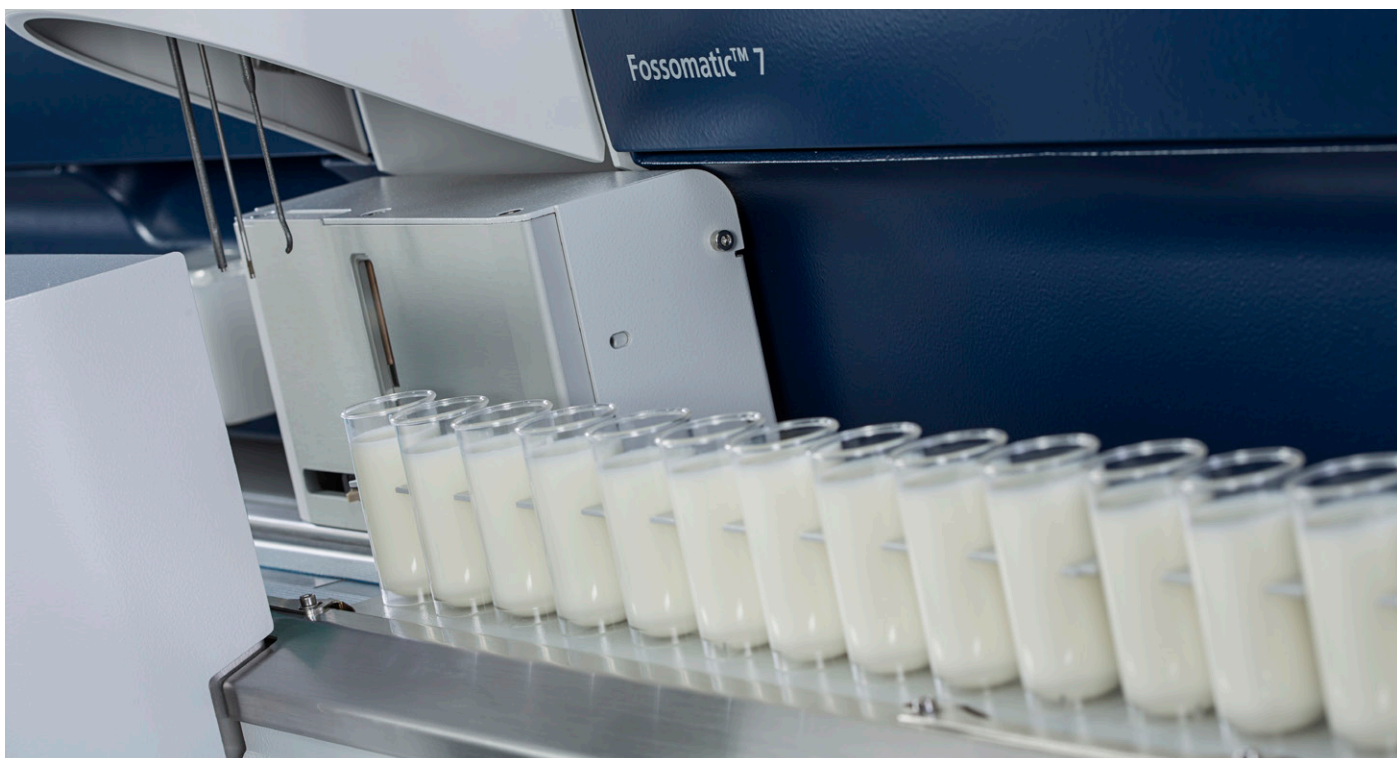
Caption: Up to 600 samples per hour handled with minimal cleaning and maintenance work
